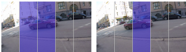
Figure 1. Left: Regions activated using the full bounding box, Right: regions activated using the bounding box center. Each region conveys 24°. Note: black vehicle is parked so it is not annotated.
