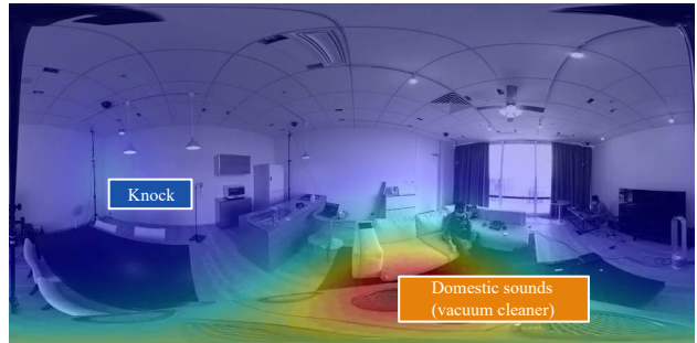
Figure 1. Still from overlay of 360° video, spatial acoustic power map generated from microphone array, and annotated event label.
